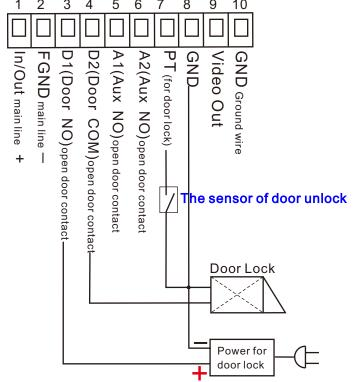
(The power of door lock must be an independent power, door phone power can't share power with door lock.)
